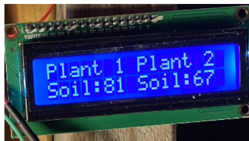
Figure 8: Outputs of the Plant 1's & Plant 2's Moisture Sensor Readings on LCD Display
